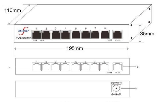
A. 8x PoE Power Port B. Uplink Port C. DC 48V Input
